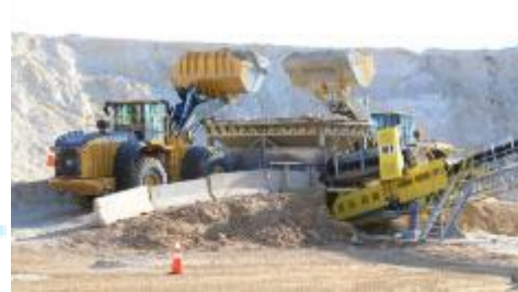
Conveyer Belt to On-site Wet Plant
