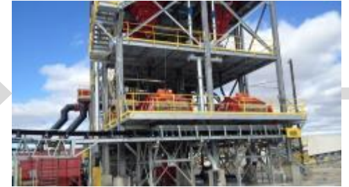
Wet Plant Cleans and Sorts Product
